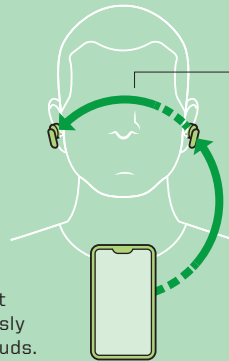
Bluetooth signal is relayed directly from the primary bud to the other bud.
